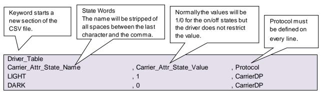
This method may be used to change the values of any of the driver's default state words by duplicating the word and specifying a new value in the configuration file.
